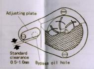
In ordinary operation , adjustment is not required for the oil pump , If oil splashing does not occur in the oil check window when the machine runs at a low speed , close the clearance of the bypass oil hole.
