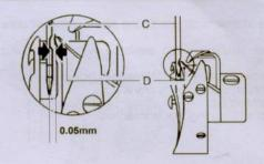
The clearance between the bottom of the needle notch and the hook tip should be  $0.05\ \text{mm}$  .
