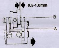
Cam Driving Crank (A), Cam (B) is seperated from the en-gagement with the roller, the standard clearance is 0.5-1.0mm.
