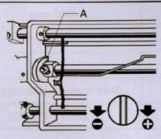
Adjust the oil amount of the rotating hook by turning the oil amount adjusting screw (A). Turn the screw (A) clockwise (in the "+" direction ) to increase the oil amount; turn it counter-clockwise (in the "-" direction ) to decrease the oil amount.
