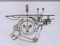
(1)When cutting thick thread, increase the cutting (2)For adjusting cutting force, loosen Set Nut (adjust Screw (B).
