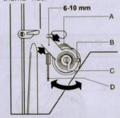
The stroke of the thread take-up spring runs from 6mm to 10mm, when sewing very thin fabrics, reduce the thread take-up spring tension and increase the thread take-up spring stroke, where as increase the thread take-up spring tension and reduce the thread take-up stroke when sewing very thick fabrics.
