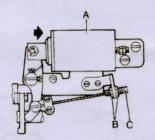
There should be a clearance of 1mm between the two discs while the thread cutting electromagnet (A) is working.
