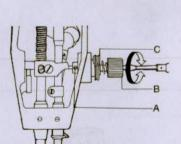
Thread tension should be determined in accordance with the stitch obtained by adjusting the tension of the bobbin thread and needle thaead.
