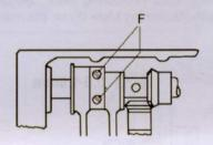
Loosen eccentric wheel screw, turn eccentric wheel and balance wheel separately to adjust the position of needle and feed doy . Then tighten the screw.
