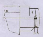
(1) Align No.2 Positioning Mark (A) on the balance wheel with Positioning Mark (B) on the machine arm.
