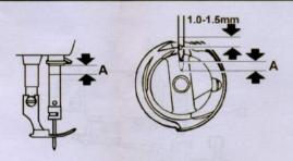
When lifting the needle bar from its lowest posi-tion of the stroke to the distance A, the hook point D of the bobbin should align with the center line of the needle and be 1.0-1.5 mm above upper end of the needle eye (Fig.15)
