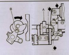
(2)As the thread cutting electromagnet works, Thread Cutting Cam (A) run in normal rotating direction. Fix the cam when Cam (A) is engaged with Roller (B).
